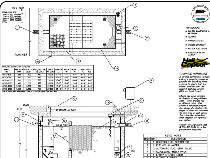
1 SLUDGE CHAMBER 6 1 DIFFUSION BAFFLE 1 HIGH FUEL ALARM PANEL 8 1 OSHA COMPLIANT SAFETY NET 10 2 4" VENT COUPLING 2 X" INPUT AND OUTPUT 11 NAMEPLATE INDICATING: 12 NAMEPLA IE INDICA IIN MFG: ParkUSA 888-611-PARK MODEL: HFSC-01 DATE MANUFACTURED 13 1 ACCESS HATCHWAY W/SAFETY NET 14 2 RESILIENT BOOT 15 1 SLUDGE BAFFLE 16 1 30 X 60 GALVANIZED STEEL PARKway. 17 | 1 | HIGH FUEL FLOAT SWITCH 18 1 3/4" CONDUIT SLEEVE
